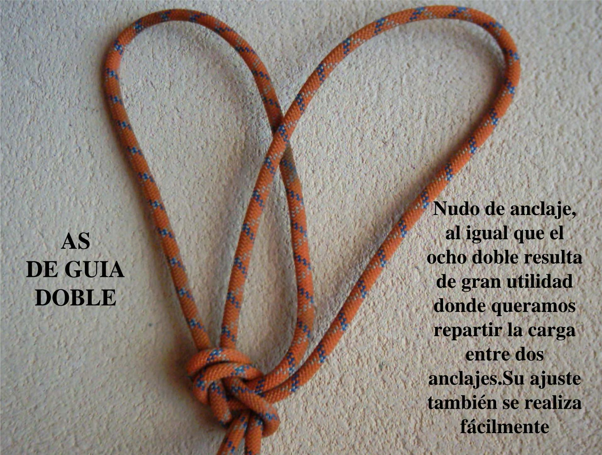
A photograph of a double anchor knot (also known as a double figure-eight knot) made from a thick, braided rope with an orange base color and blue and white speckles. The knot is shown against a light-colored, textured background. The rope forms two large, symmetrical loops that meet at a central point where the knot is tied. The knot is designed to distribute weight evenly between two anchor points.
